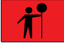
Traffic Controller ahead, be prepared to stop.
